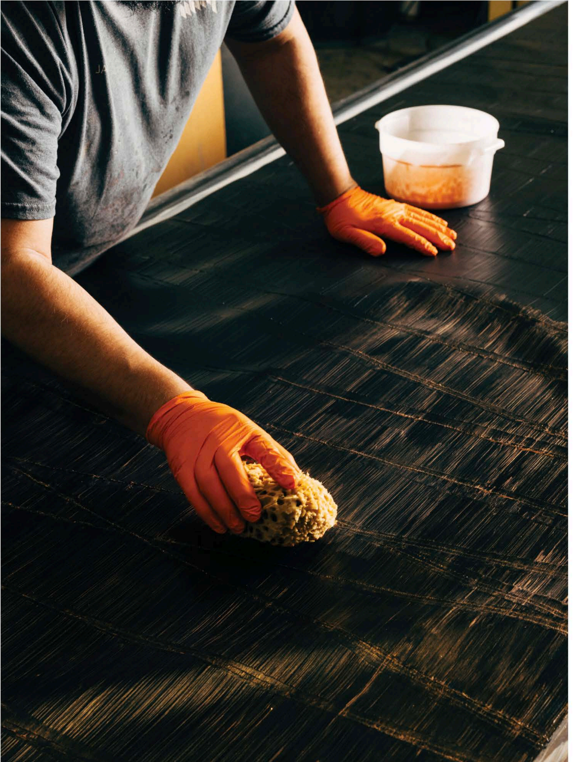
"At first I mixed the metallic into the color itself. Now we have changed to the faster way: we spray the color, and then we do a little metallic accent on top," Bo says. Left, the base color is applied. Above, a quick sponge touch adds the metallic tipping.
