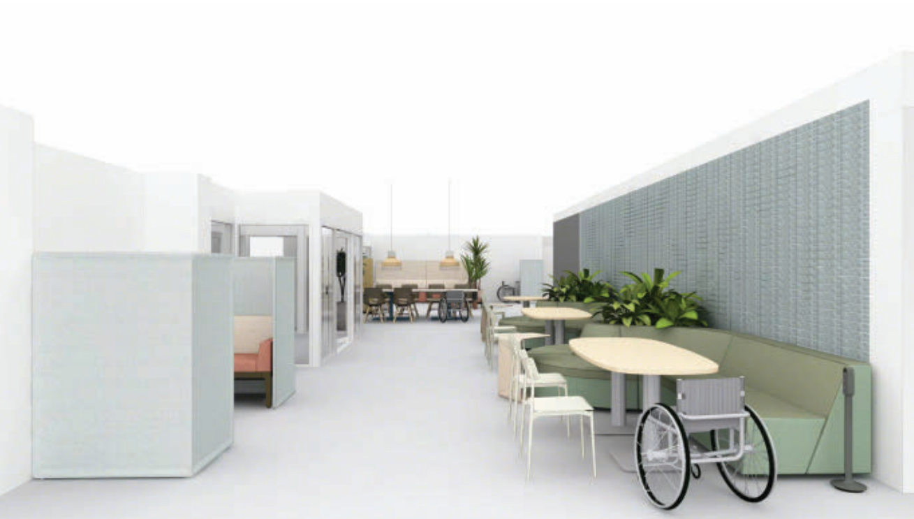
Breakout spaces concept: Acoustic tiles applied to the wall help dampen sound, important for those who might get over-stimulated or struggle to isolate voices. Lounge seating serves as a landmark while chairs and personal tables can be moved as needed. Shielded spaces allow for individual privacy or small private group conversations.
